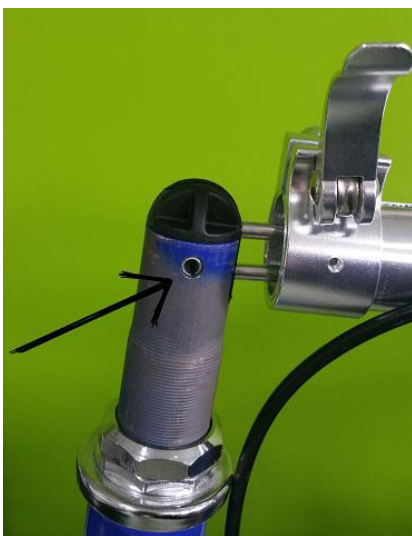
You need to remove the locking bracket (see arrow).
