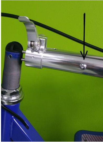
This bolt needs to be loosened so the folding guidance can be taken out of the steering tube.
