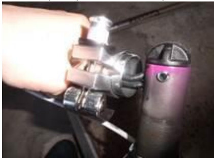
You can see the folding guidance is bent.
